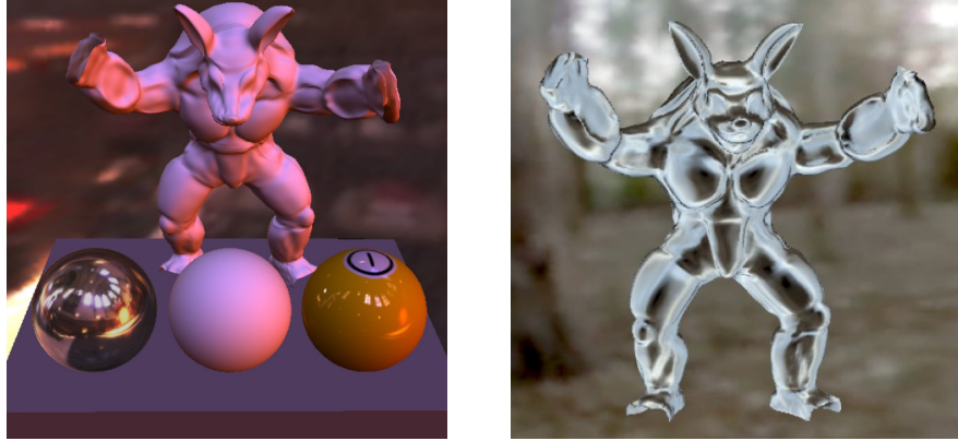
Fig. 3.6 Spherical harmonic methods used for environment map rendering, based on the reflection as convolution framework. On the left, Lambertian and mirror reflections, along with standard diffuse textures, rendered using the nine term model for irradiance [108]. On the right, we show general materials (in this example, an anisotropic reflection model), using the convolution formula for general BRDFs [111]. These scenes can be rendered in real-time with environment maps. The techniques involved would not usually be classified as precomputation-based methods, since minimal precomputation is required and the scene geometry can be changed dynamically. However, these methods also do not include cast shadows or interreflections, as in modern PRT methods.
